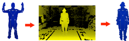
Figure 5: Our Kinect calibration pose (left), applied to the pre-recorded depth map for Anne-c1-t1 (centre), giving a skeletal overlay (right).
