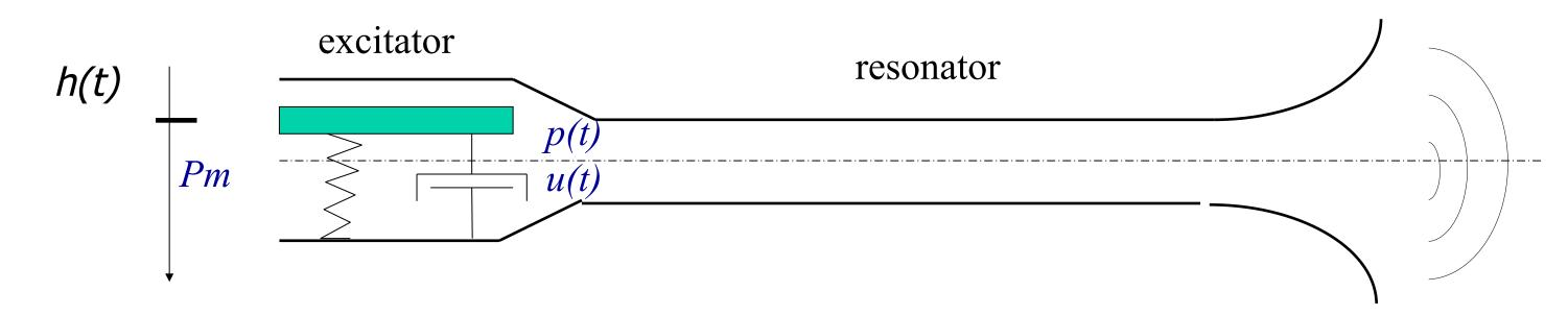
Coupling of a non-linear excitator (characterized by mechanical parameters) with a linear resonator (characterized by the input impedance  $Z_{in}$ )
